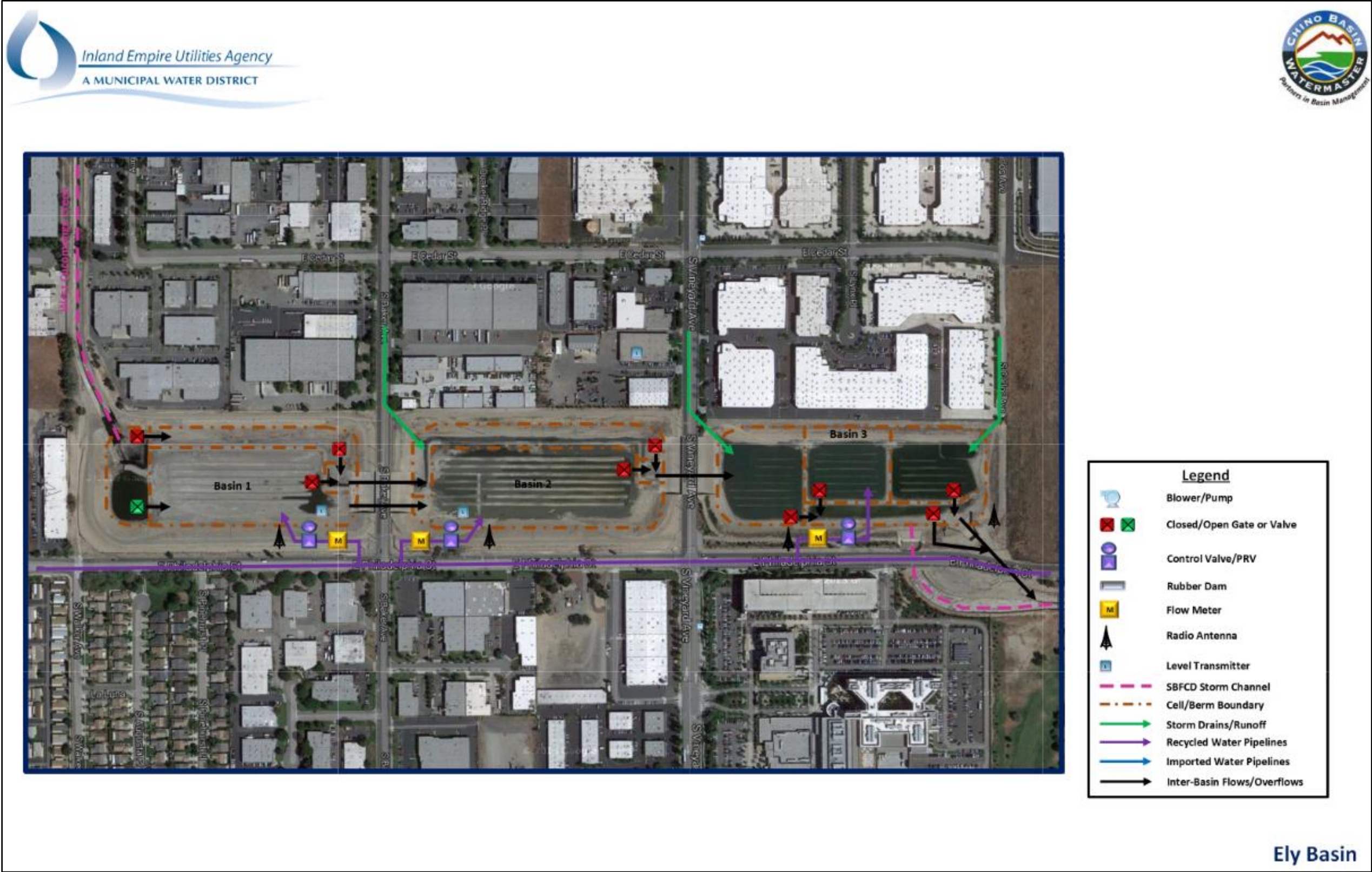
Figure 7-42 Ely Basin (GRW) Process Flow
