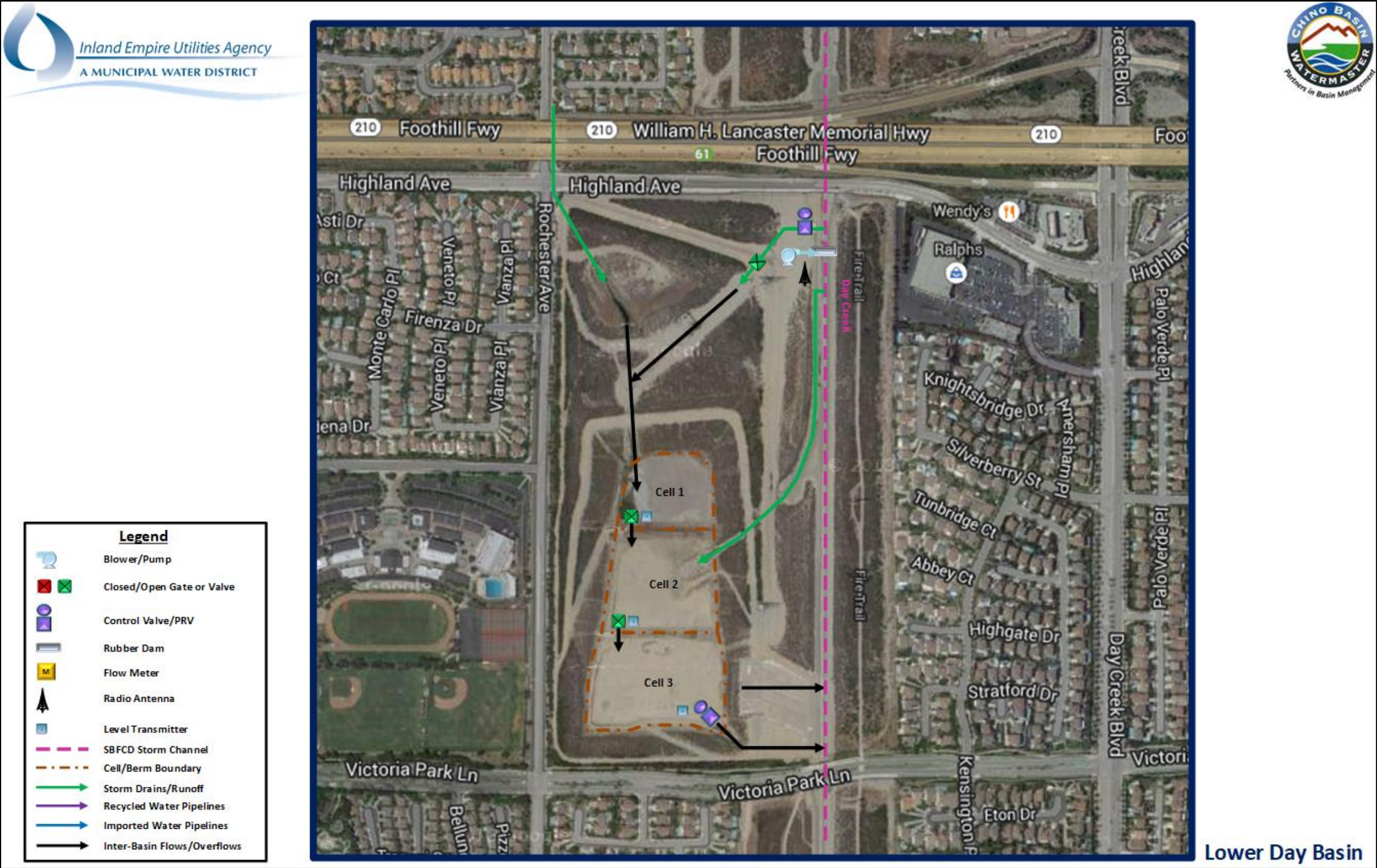
Figure 7-47 Lower Day Basin (GWR) Process Flow
