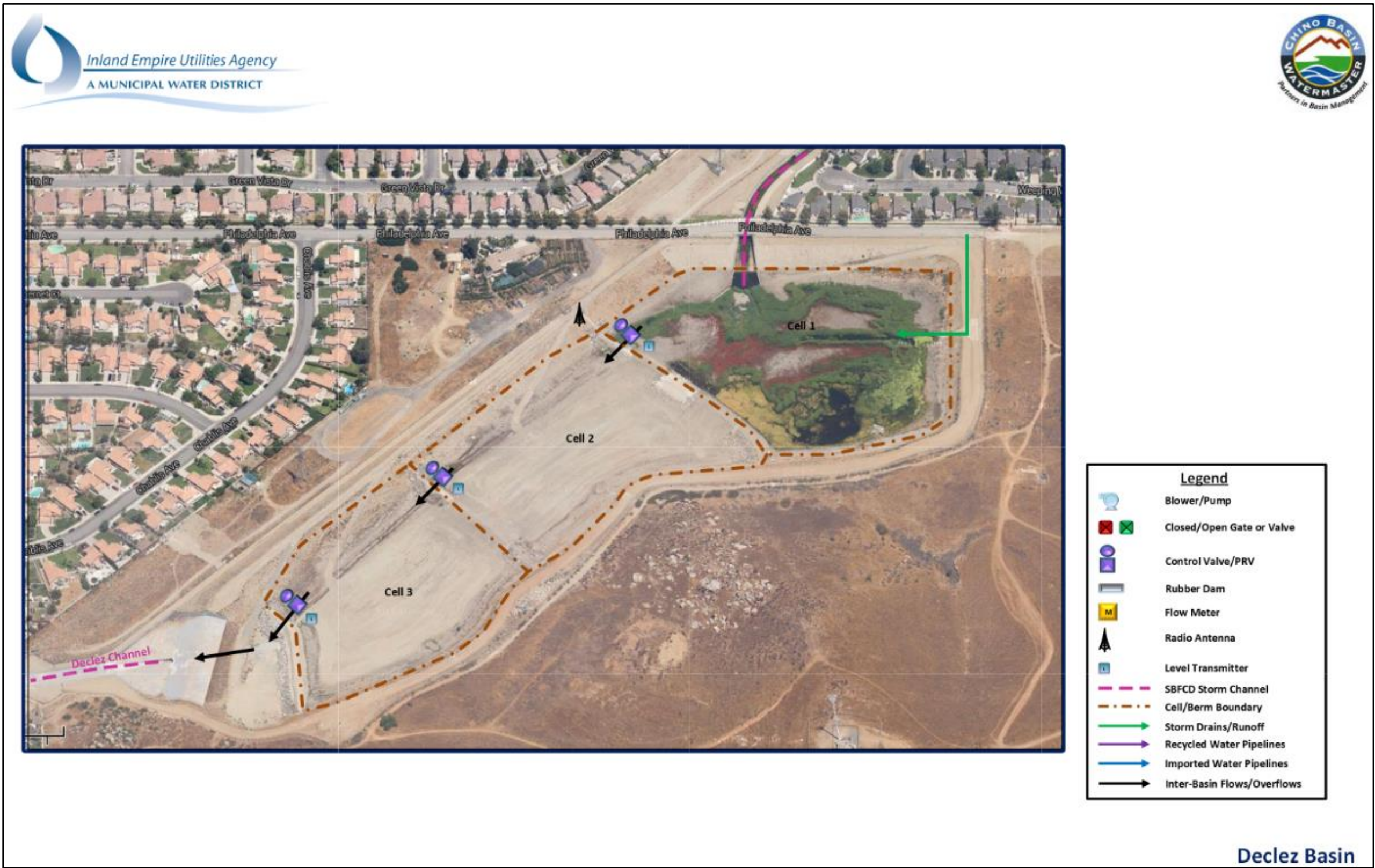
Figure 7-41 Declez Basin (GWR) Process Flow
