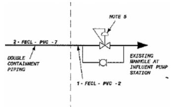
Figure 3-9: Ferric Chloride Dose Location
