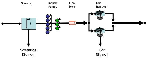
Figure 1 – Preliminary Treatment Process Schematic
