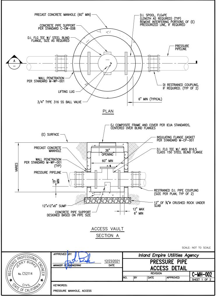
G:\EN/1-Engineering Standard Details/Progress Standard Details/Files to add signature/CAD/Phase 1/C-MH-002.0wg Dec 23, 2021 - 10:14am
