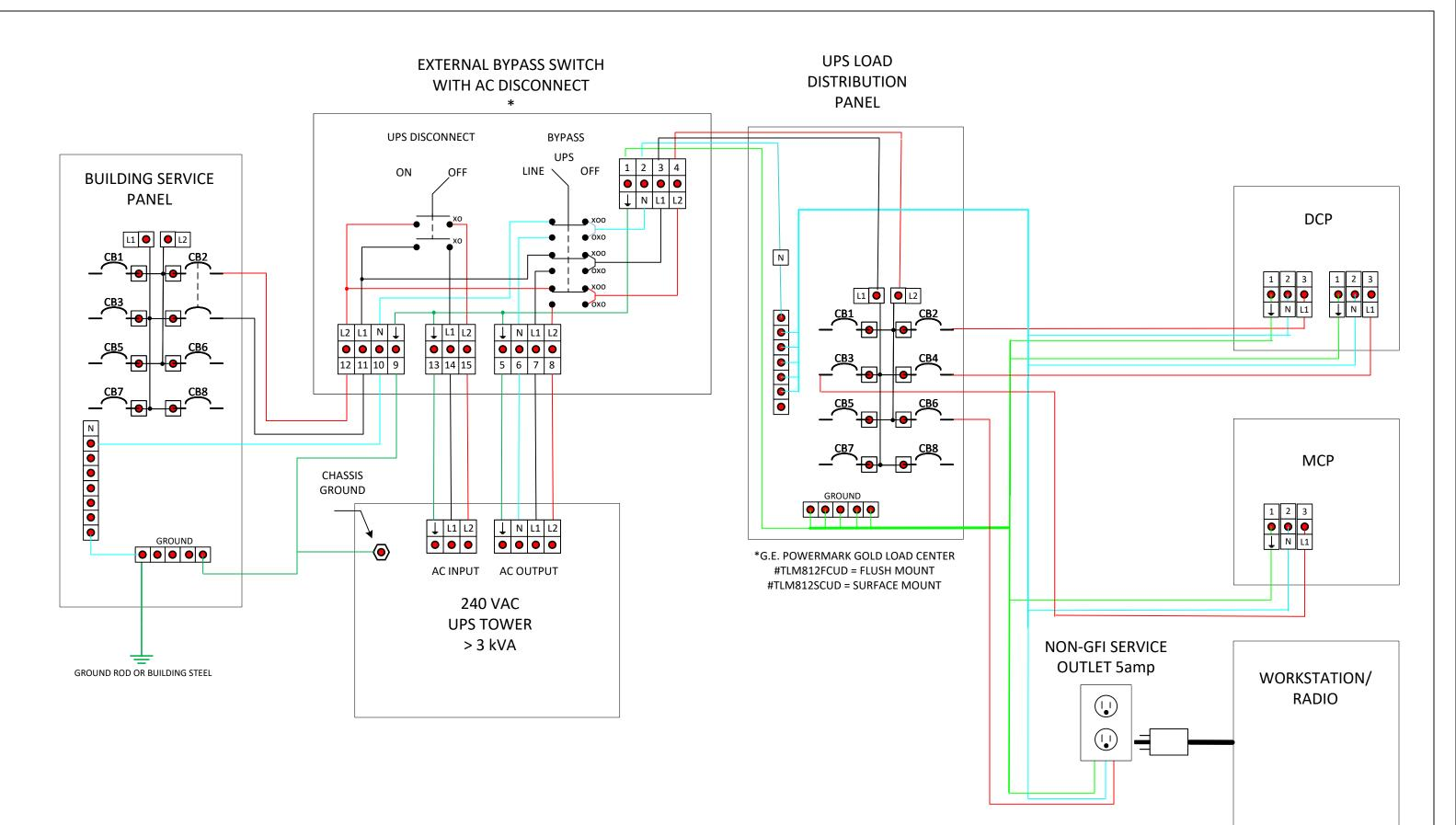
\*EATON Bypass Switch BPE02MBB1A - (240 VAC up to 7kVA) BPE04MBB1A - (240 VAC up to 12.5 kVA) BPE05MBB1A - (240 VAC up to 18 kVA)
