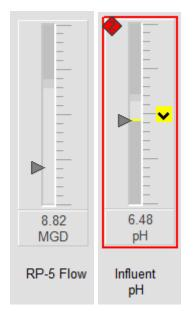
Figure 9: Typical Analog Indicator
