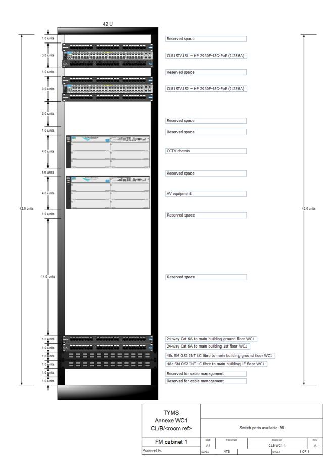
*Figure 3.* Example of layout diagram for a "Facilities Management" cabinet in a major wiring center, accommodating third-party equipment and associated fiber optic panels.
