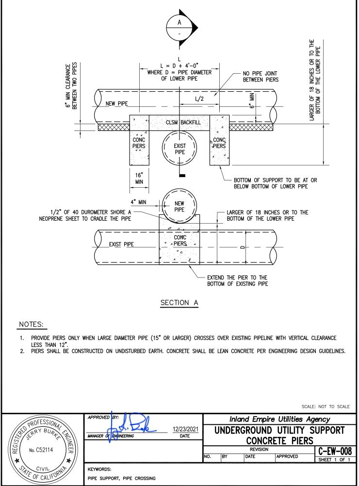
G:\EN\1-Engineering Standard Details\Progress Standard Details\Files to add signature\C4D\Phase 1\C-EW-008.dwg Dec 23, 2021 - 9:54am
