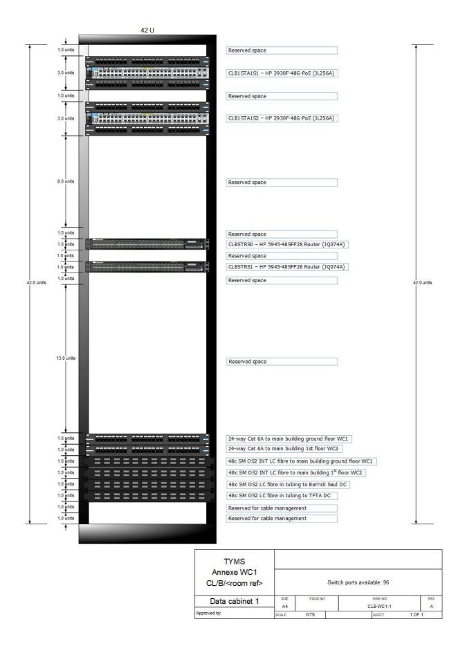
*Figure 2.* Example of layout diagram for the first cabinet in a major wiring center, accommodating two chassis switches for network routing, and several fiber optic panels.
