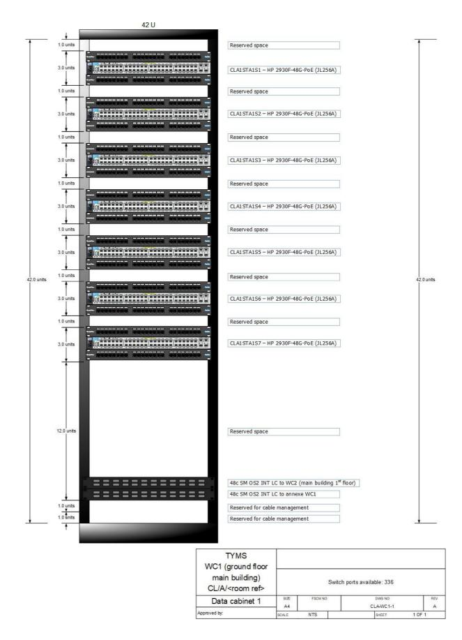
*Figure 1.* Example of standard cabinet layout diagram, accommodating 14 patch panels and up to 336 data outlets; space has been left for more sets.
