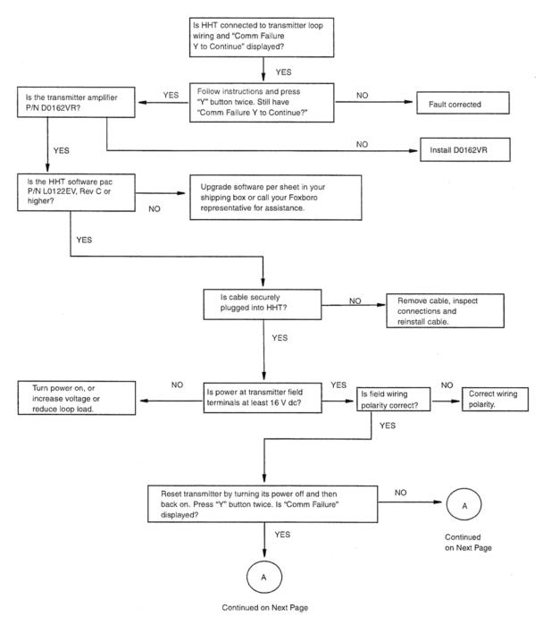
Figure 43. Communication Failure Flowchart
