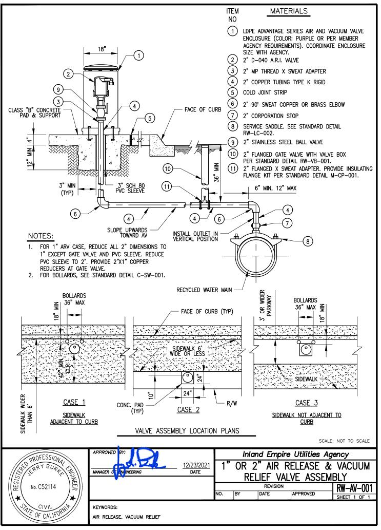
G\EN\1-Engineering Standard Details\Progress Standard Details\Files to add signature\C4D\Phase 2\RW-AV-001.dwg Dec 23, 2021 - 3:16pm
