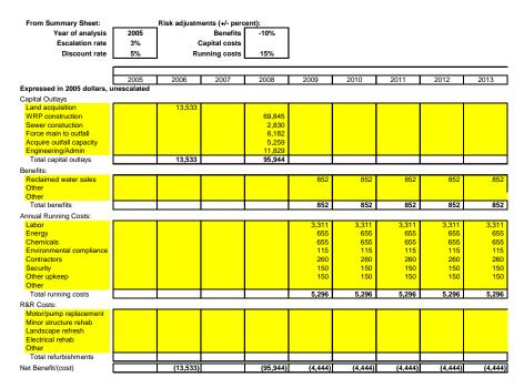
Figure 5: Partial NPV Tool, Example of Data Entry with Sensitivity Adjustments
