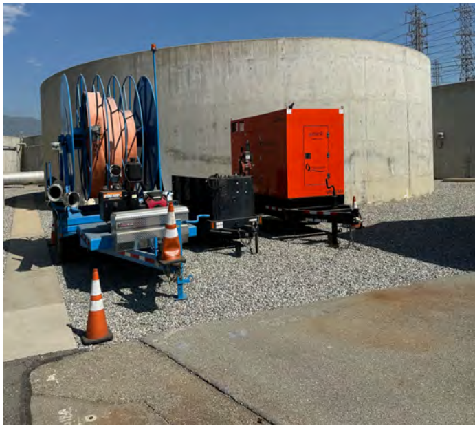
Task D (Photo D7): Inspection lay-flat hose trailer, generator, and other emergency spare equipment.
