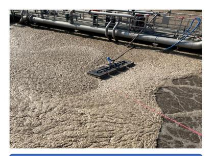
OTE testing and Analyzer set up at RP-4
