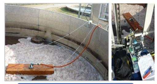
Off-gas testing and Analyzer set up at RP-4
