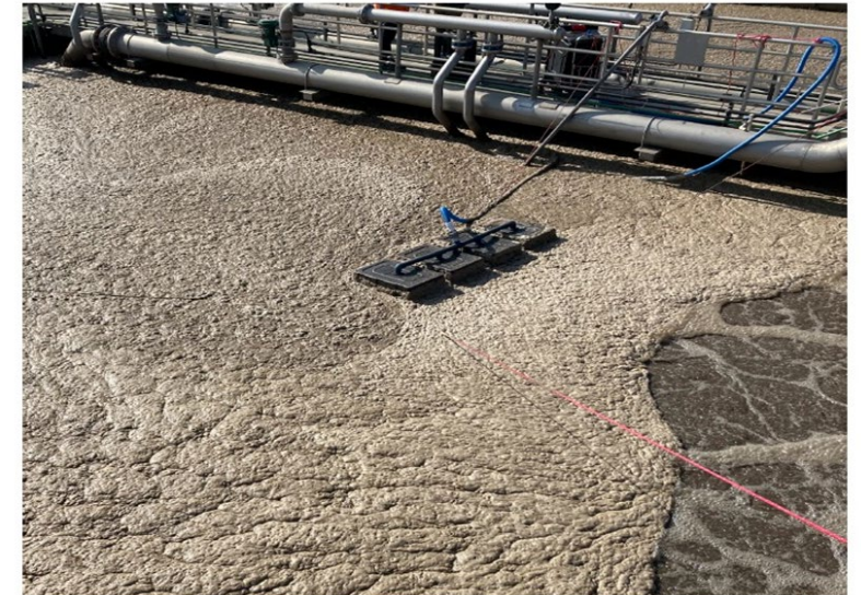
OTE testing and Analyzer set up at RP-4
