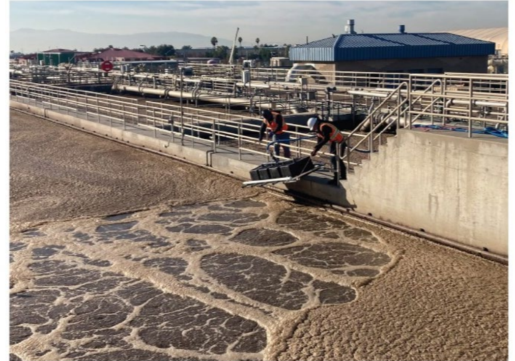
Dr. H2O's crew performing OTE gas collection at Aeration basin Train 3 on 12/16/2021
