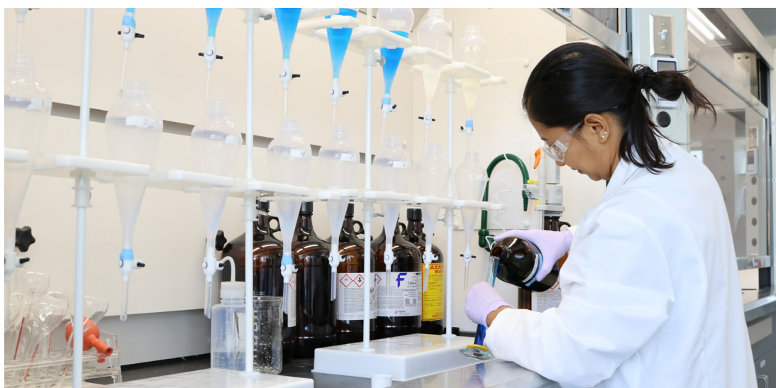
Quality Control Analyst performing Sulfonates testing, a methylene blue color reaction to detect the existence of anionic substances in water that may cause water corrosion or contamination.
