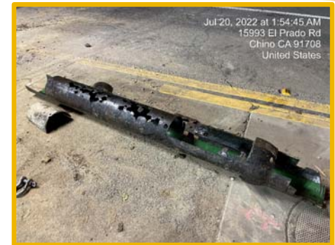
8-foot of Corroded Pipe Removed
