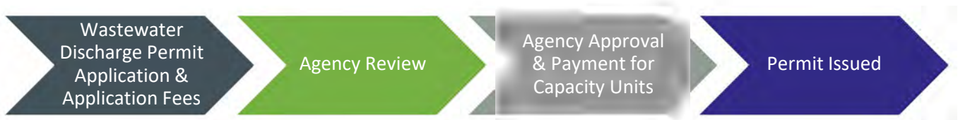
Figure 2-1. Typical Process for Wastewater Discharge Permit
