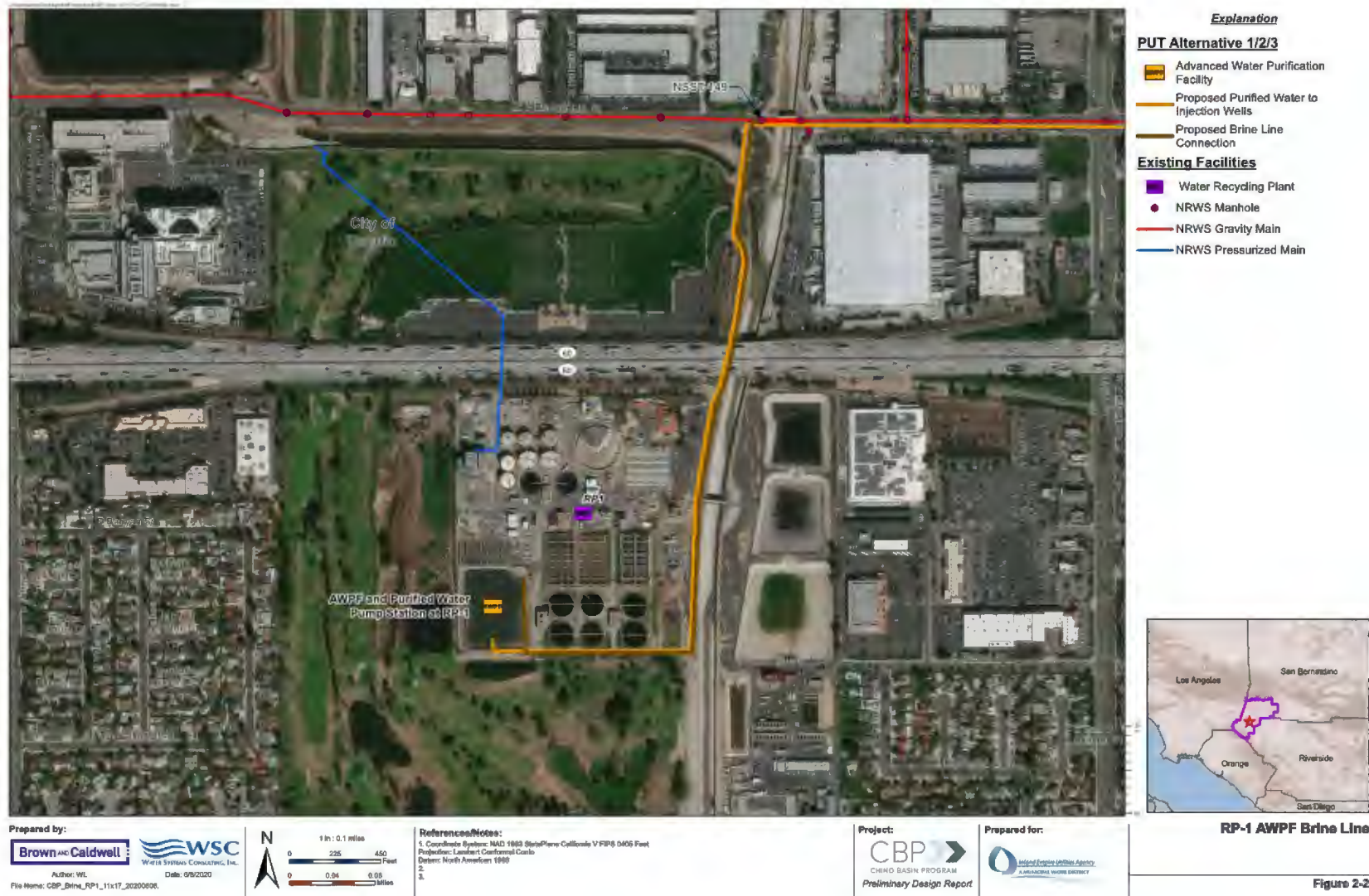
Figure 2-2. RP-1 AWPB Brine Line
