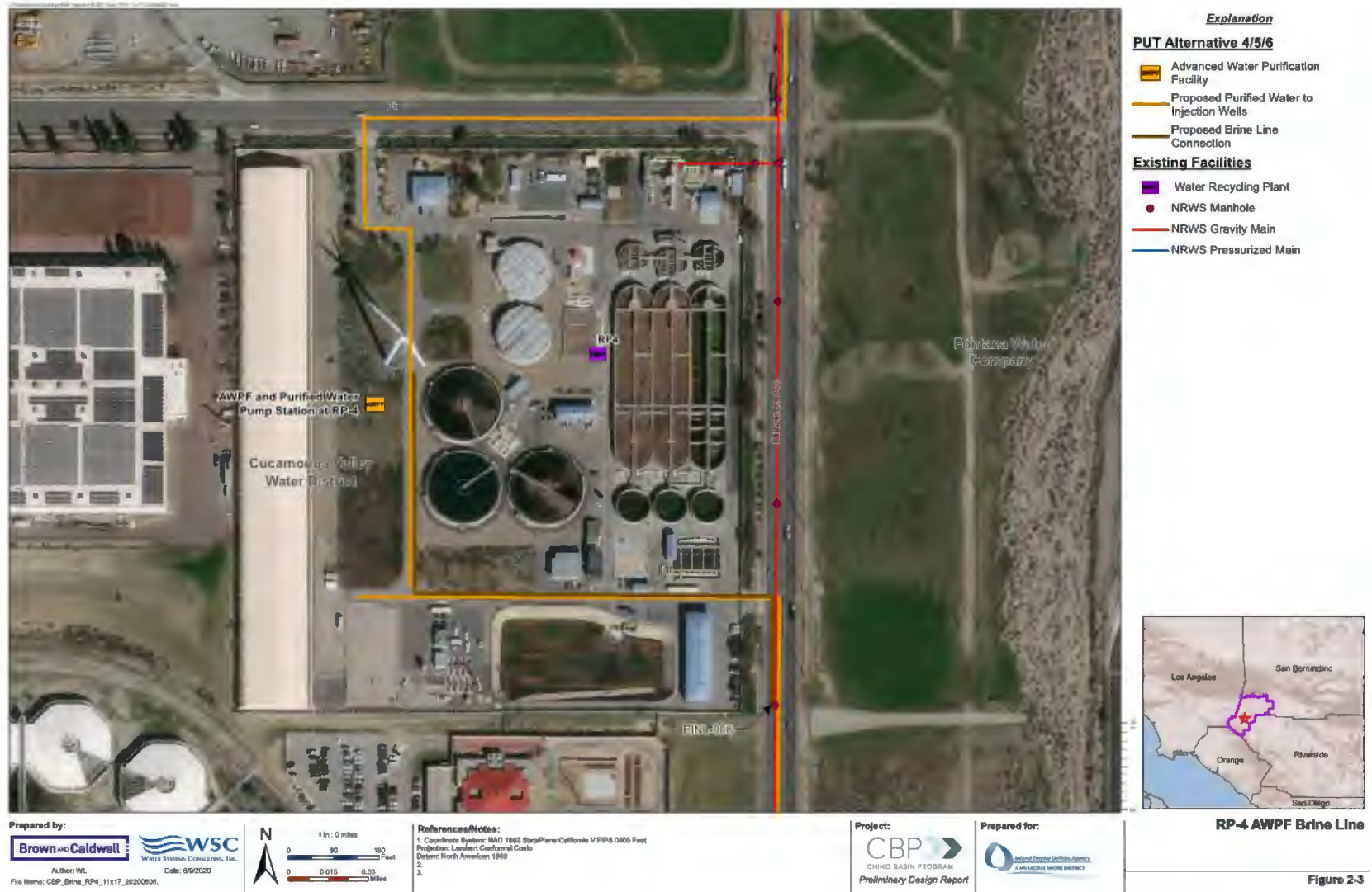
Figure 2-3. RP-4 AWPB Brine Line
