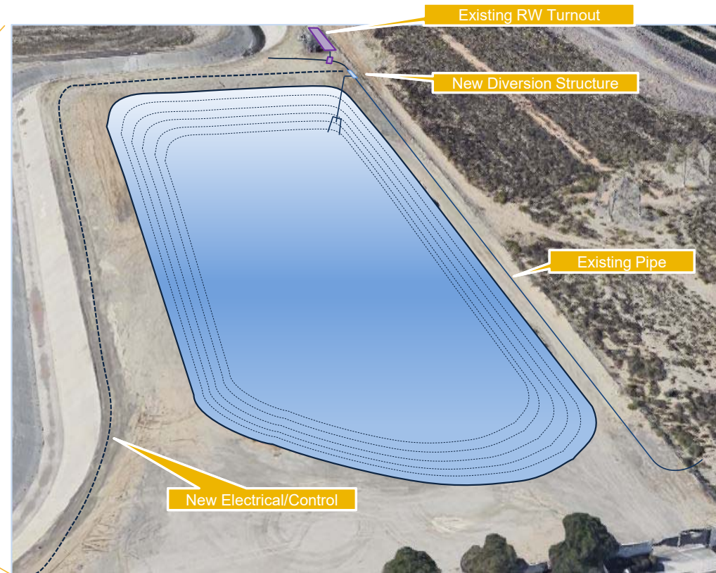
Sketch of Completed New Basin Over Abandoned Structures
