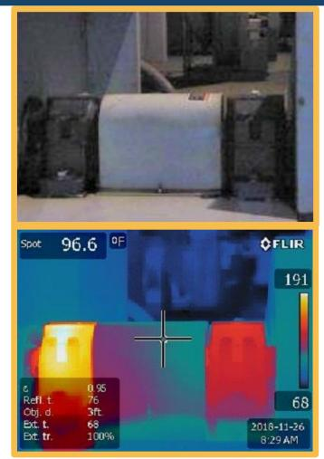
Normal photo vs. thermal image of over-heating bearing
