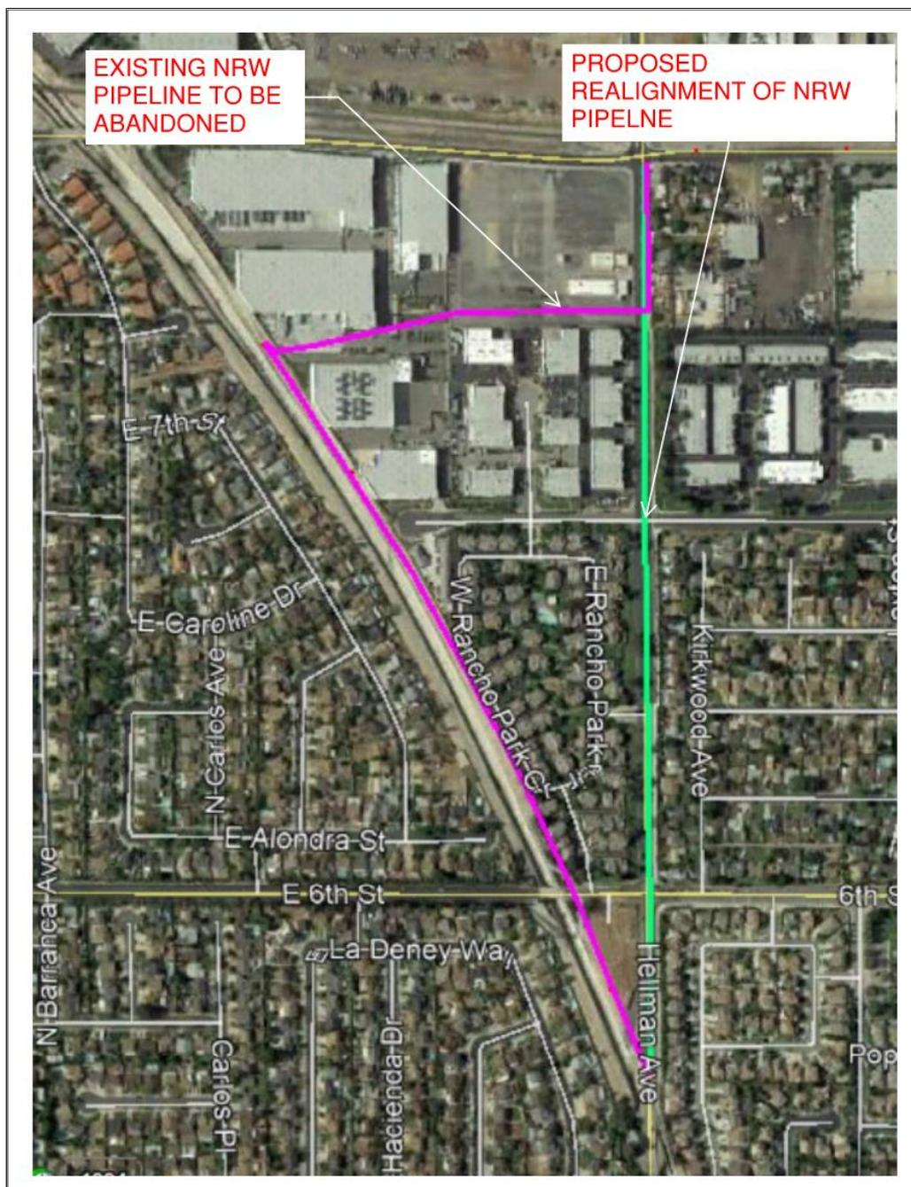
Figure 1: Pipeline Alignments
