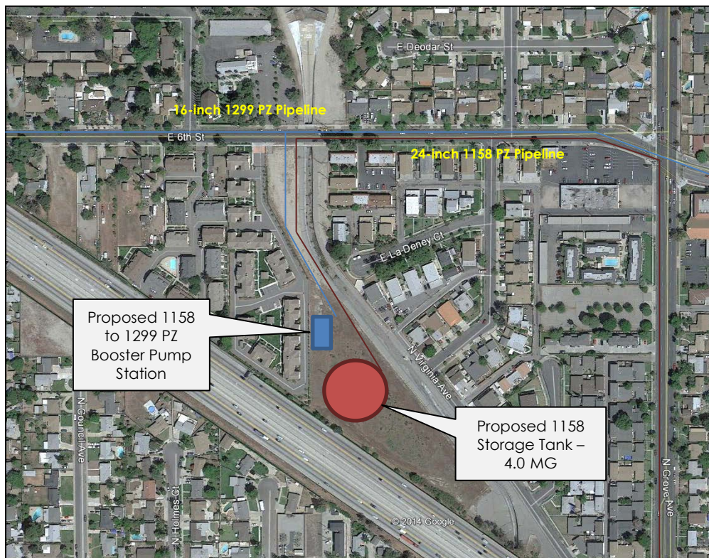
Figure 6-2 Proposed 1158 Storage Tank Site
