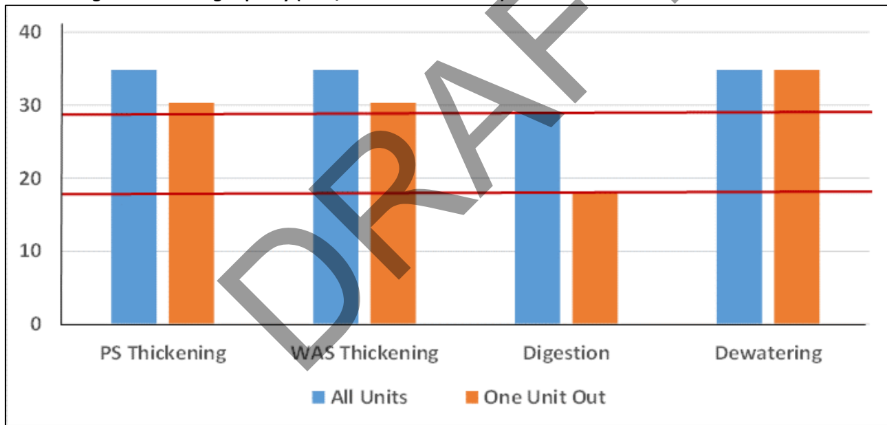
FIGURE 7-5 RP-2 Existing Solids Handling Capacity (RP-5/CCWRF Waste Solids)
