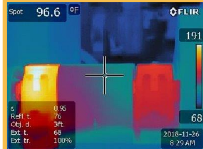
Normal photo vs. thermal image of over-heating bearing
