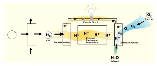
**Figure 4-6: Fuel Cell Power Generation Process**
