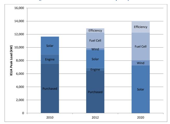
Figure 4-3: Peak Period Electrical Load Gap Analysis
