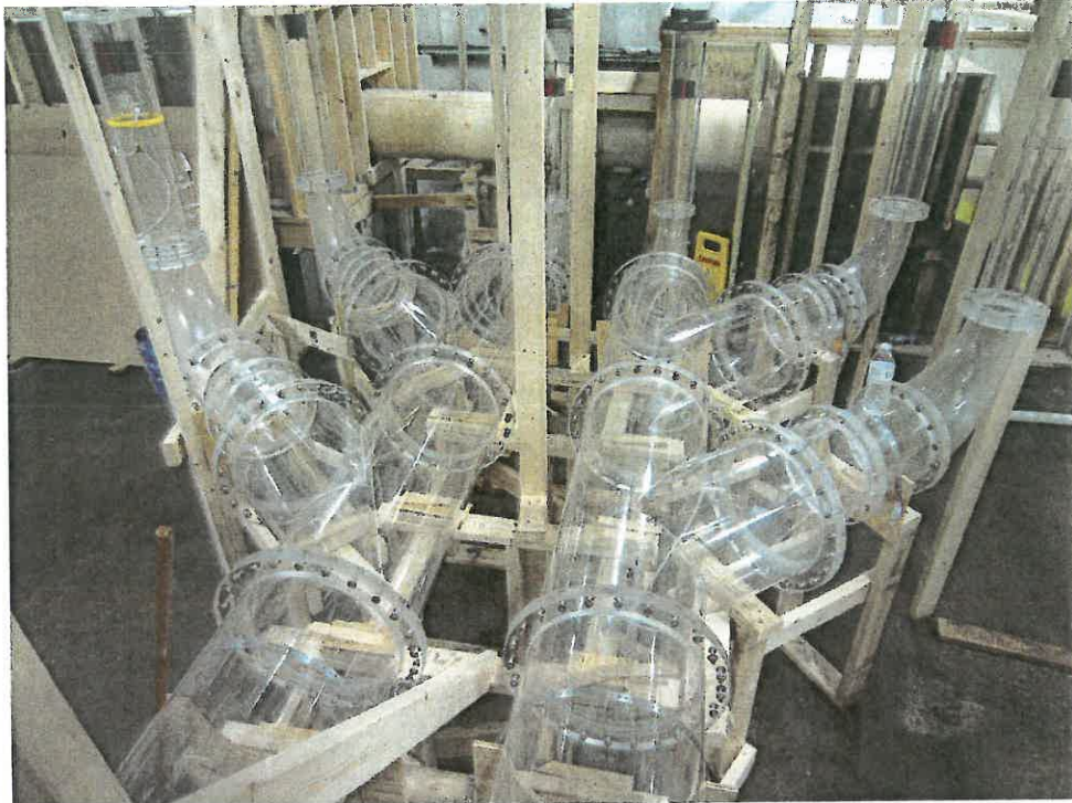
Photo 6 All Pumps Will Be Made In-House from Clear Acrylic for Full Flow Visualization
