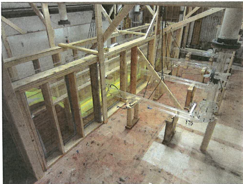
Photo 3 CEH Can Model Both Horizontal and Vertical Pumps With This Style Intake
