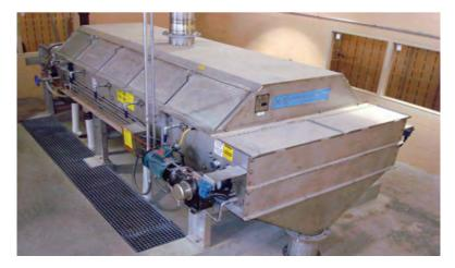
Figure 7.3-8: Gravity Belt Thickener
