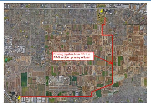
Figure 9-9: RP-1 to RP-5 Gas Pipeline – Potential Alignment
