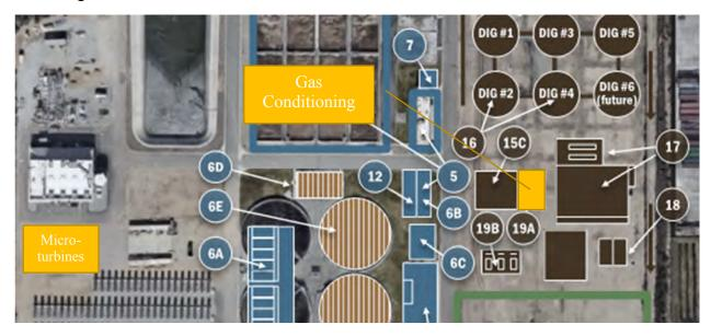
Figure 9-8: Alternative 2 – Proposed Site Layout
