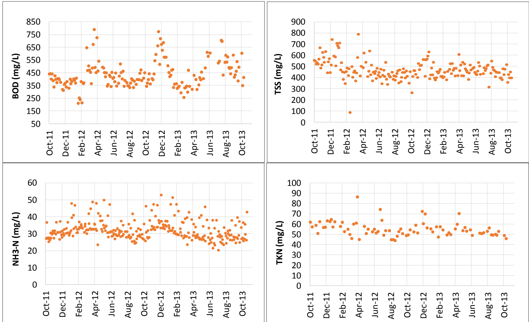
FIGURE 4-5 RP-1 Influent Wastewater Quality
