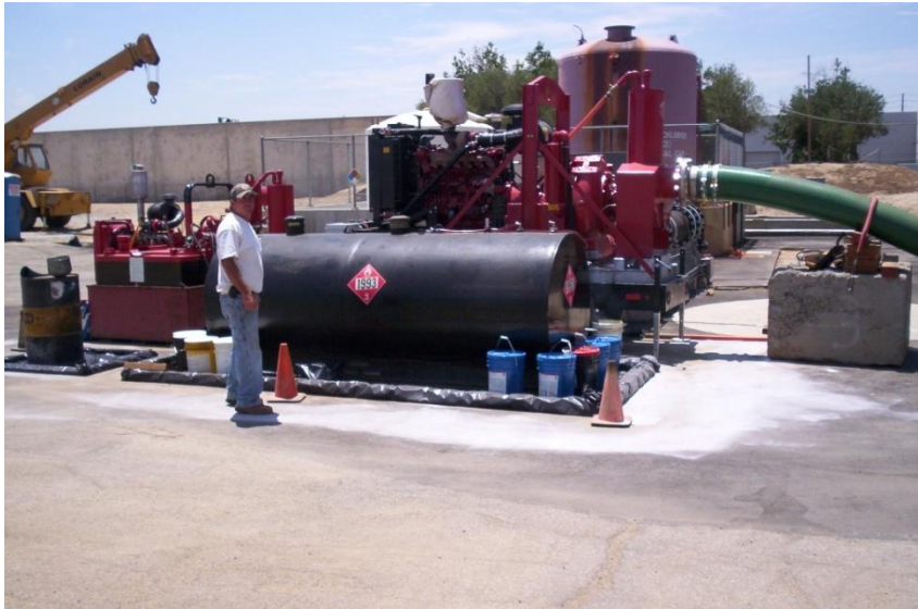
NRWS Philadelphia Pump Station (Engine Driven Bypass Pump)
