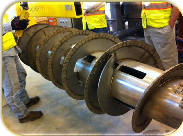
RP-1 Dewatering Expansion Project Alfa Laval's G2-120 Centrifuge Scroll
